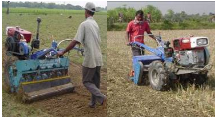
Photograph 1: PTOS in operation in fallow land (left) and in the left-over residue plot (right) after Aman rice harvest
